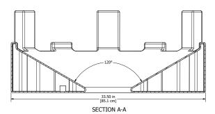
The SSOP-400/600 Support Stand is a one-piece construction with a conical module that sits on the floor. For use with Trapzilla models TZ-400 and TZ-600. It does not add appreciable height to the assembly.
