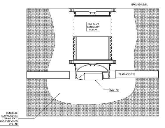
In order to offset the effects of buoyancy caused by groundwater (high water tables), Thermaco, Inc. recommends concrete be poured around the anchor ring and the Trapzilla<sup>®</sup> installed inground. The amount of concrete to be used is specified in the table below. The concrete is to be poured continuously and completely surrounding the Trapzilla<sup>®</sup> body (and Extension Collars if applicable) to ensure proper strength and security.
