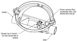
The TZSP-40 has no vertical fall, so the jar must be turned horizontally to catch the flow. The patent pending flume accelerates flows, allowing horizontal sample filling despite the lack of a substantial fall.
