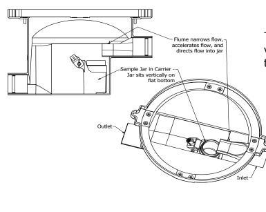
To sample the TZSP-48, leave the jar sitting vertically so it may catch the vertical flow of the water as it flows out of the flume.
