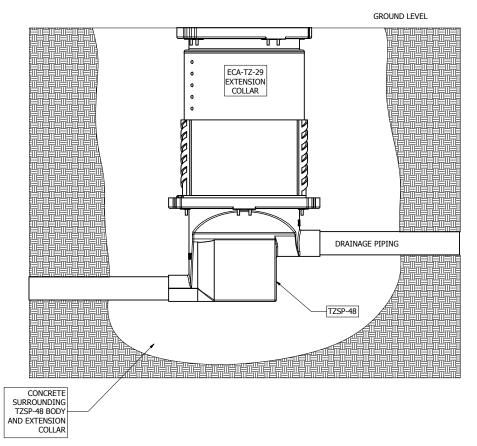
In order to offset the effects of buoyancy caused by groundwater (high water tables), Thermaco, Inc. recommends concrete be poured around the anchor ring and the Trapzilla<sup>®</sup> installed inground. The amount of concrete to be used is specified in the table below. The concrete is to be poured continuously and completely surrounding the Trapzilla<sup>®</sup> body (and Extension Collars if applicable) to ensure proper strength and security.
