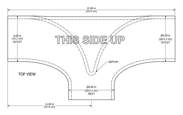
**Material: Rotationally Molded Polyethylene**
