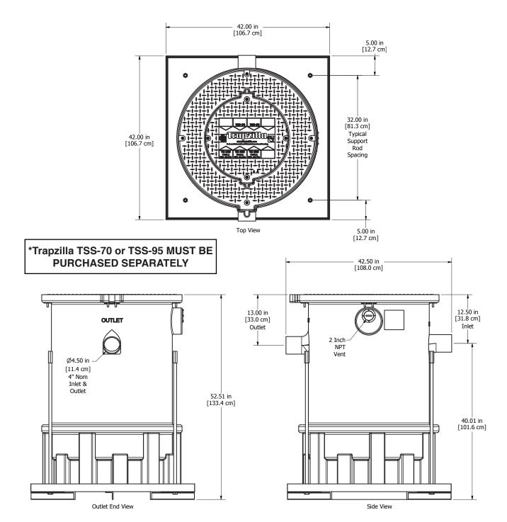
Thermaco, Inc. supplies the frame & support base with the HA-70/95. This include four (4) 36" threaded rods and the nuts to connect to a contractor-installed, in-floor suspension mount. This kit needs to be installed by a licensed contractor. The contractor is responsible for determining weight loads, preparation of the floor for installation and any construction necessary for installation of the suspension kit.
