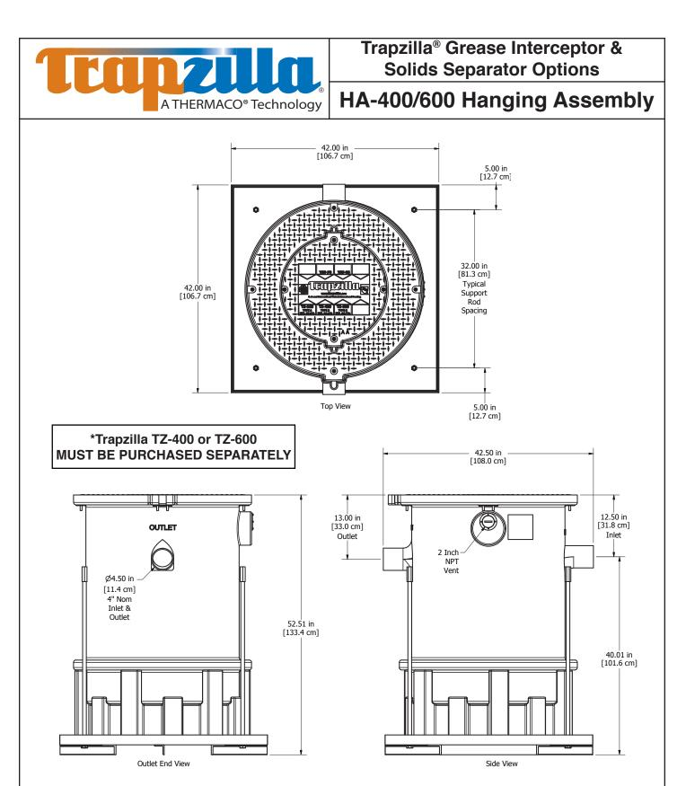
Thermaco, Inc. supplies the frame & support base with the HA-400/600. This include four (4) 36" threaded rods and the nuts to connect to a contractor-installed, in-floor suspension mount. This kit needs to be installed by a licensed contractor. The contractor is responsible for determining weight loads, preparation of the floor for installation and any construction necessary for installation of the suspension kit. <u>One SSOP-400/600 Support Frame comes with the HA-400/600</u>.
