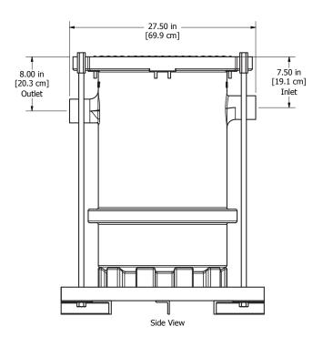
Thermaco, Inc. supplies the frame & support base with the HA-160. This include four (4) 36" threaded rods and the nuts to connect to a contractor-installed, in-floor suspension mount. This kit needs to be installed by a licensed contractor. The contractor is responsible for determining weight loads, preparation of the floor for installation and any construction necessary for installation of the suspension kit.
